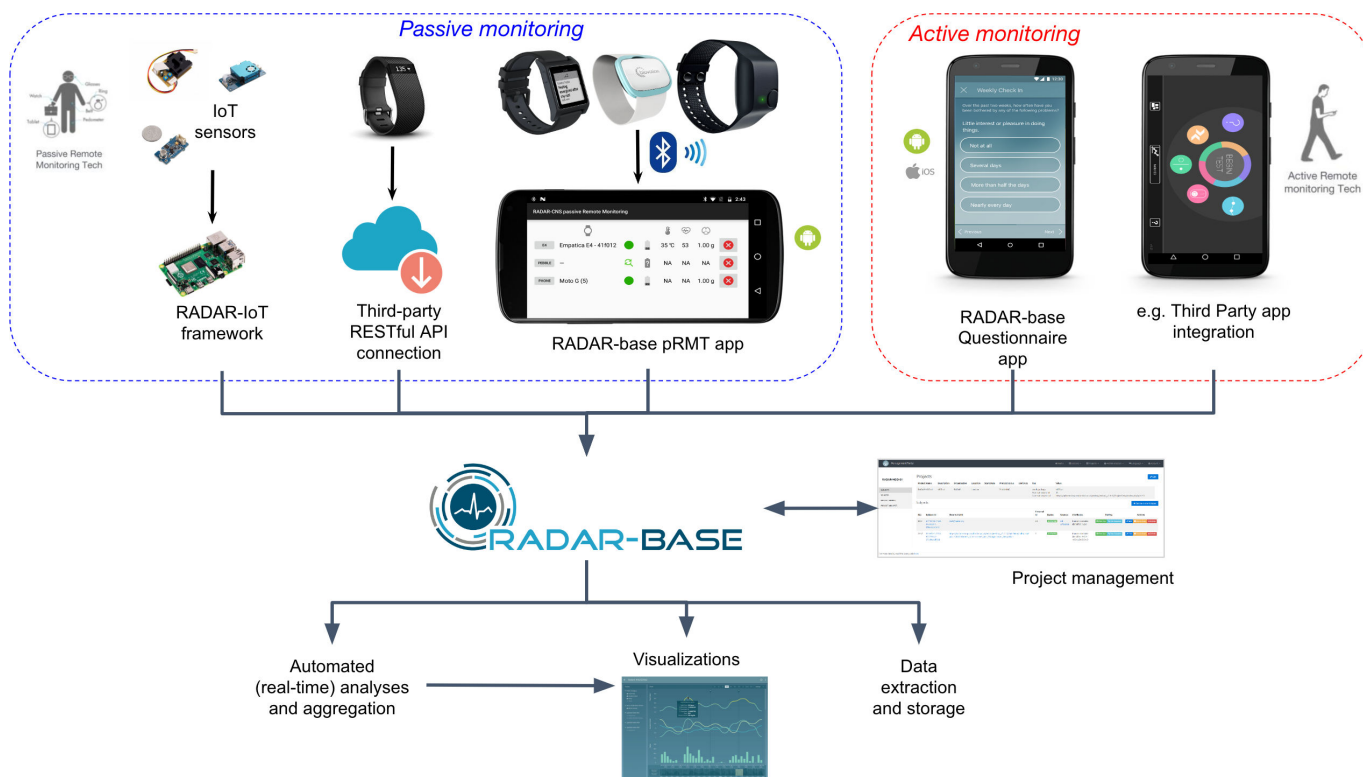
Figure 1. Overview of the RADAR-base platform. Current data sources: Empatica E4, Pebble 2, Fitbit, Biovotion, Faros, Garmin, Active Remote Monitoring questionnaire app and Passive Remote Monitoring app. API: application programming interface; IoT: Internet of Things.
