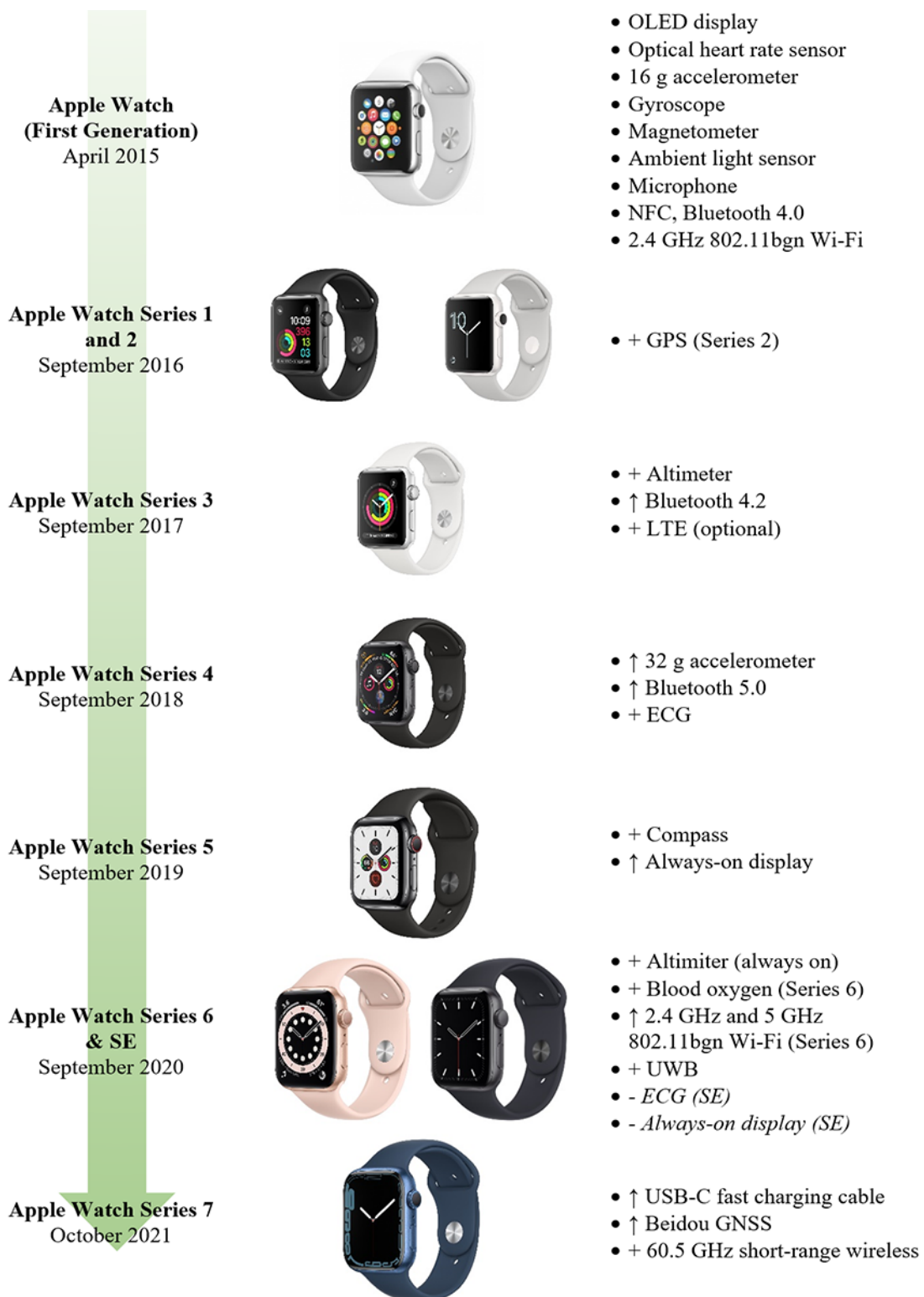
Figure 2. Evolution of Apple Watch Series features. Feature upgrades (↑) and new feature additions (+) are indicated. ECG: electrocardiogram; GNSS: global navigation satellite system; LTE: Long-Term Evolution; NFC: near-field communication; OLED: organic light-emitting diode; UWB: ultrawide band.
