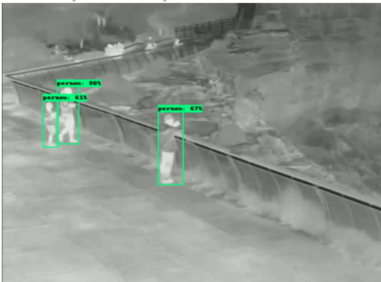
Figure 10. Pedestrian Identification using Thermal Cameras. The output of the EfficientDet pedestrian detection algorithm using data from a thermal camera. Individuals in the foreground are shown within bounding boxes with confidence levels between 61-80%.
